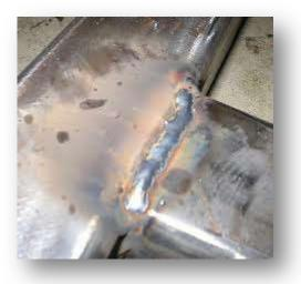
Welding is the process of joining 2 metals together by heating them up to molten hot temperatures, and then manipulating the molten weld puddle to create a weld bead.
