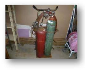
acetylene which produces a flame that burns very hot.
