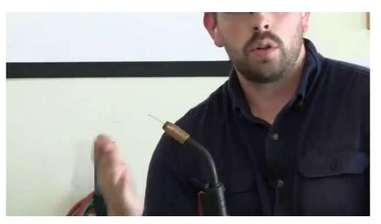
MIG welding is similar to stick welding in that you must ground the work piece with the ground clamp before you start the weld. The process of MIG welding is much faster than stick welding because you have a continuous wire being fed, and you don't have to stop and change out spent electrodes.
