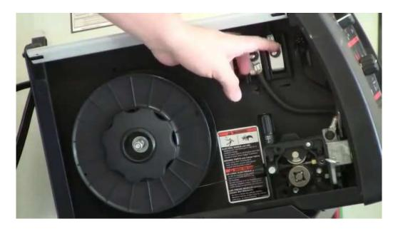
You can see the wire spool in this image, and if you look closely you'll see the wire being fed into the rollers. Once it reaches the end of the MIG gun, it melts and becomes the actual weld bead.
