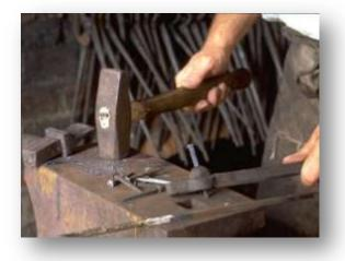
This process fused the metal together, and it's called forge welding. Up until the mid-1800's most welding was done this way.
