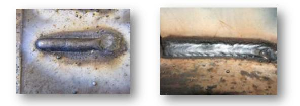
Unlike the MIG (Metal Inert Gas, a.k.a. GMAW) process, the flux core arc welding process can be used in windy conditions because there is no shielding gas to get blown away.
