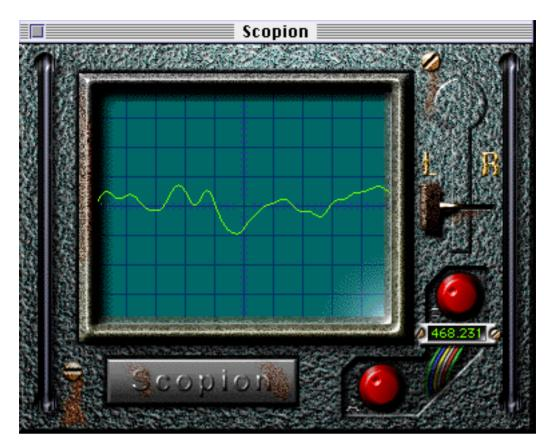
The Scopion is an on-board oscilloscope, that analyzes the left or right side of a stereo input signal and displays the waveform contents in real time. It must be used as a Master Effect. Since the Scopion uses a custom interface, you have to click the Edit button in the Master Effects window to use it. There are three parameters:
