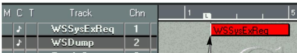
This Part contains the request message. When it is played back it makes the instrument transmit a dump...
