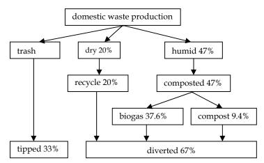
Fig. 1. Material movement of domestic waste at threshold situation
