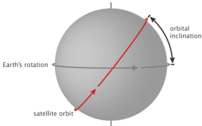
Orbital inclination is the angle between the plane of an orbit and the equator. An orbital inclination of  $0^\circ$  is directly above the equator,  $90^\circ$  crosses right above the pole, and  $180^\circ$  orbits above the equator in the opposite direction of Earth's spin. (NASA illustration by Robert Simmon.)
