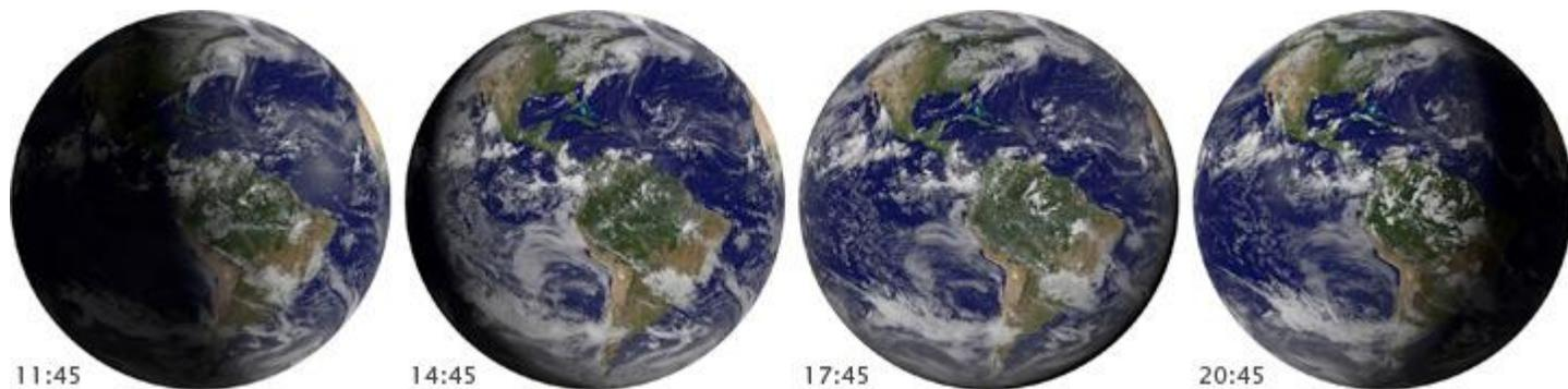
Satellites in geostationary orbit rotate with the Earth directly above the equator, continuously staying above the same spot. This position allows satellites to observe weather and other phenomena that vary on short timescales. (NASA images by Marit Jentoft-Nilsen and Robert Simmon.)
