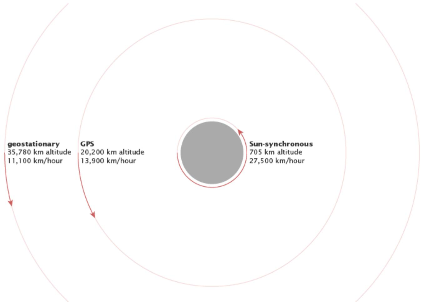
The higher a satellite's orbit, the slower it moves. Certain orbital altitudes have special properties, like a geosynchronous orbit, in which a satellite travels around the Earth exactly once each day. The length of each red arrow in this diagram represents the distance traveled by a satellite in an hour. [View animation.](#) (NASA illustration by Robert Simmon.)
