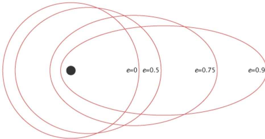
The eccentricity ( $e$ ) of an orbit indicates the deviation of the orbit from a perfect circle. A circular orbit has an eccentricity of 0, while a highly eccentric orbit is closer to (but always less than) 1. A satellite in an eccentric orbit moves around one of the ellipse's focal points, not the center. (NASA illustration by Robert Simmon.)
