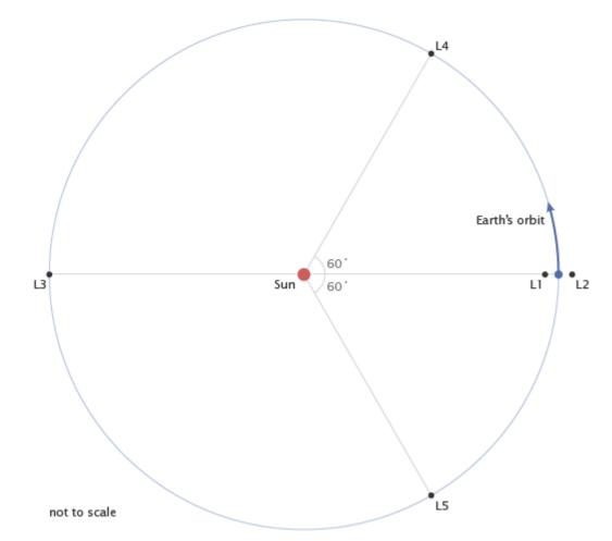
Lagrange points are special locations where a satellite will stay stationary relative to the Earth as the satellite and the Earth revolve around the Sun. L1 and L2 are positioned above the day and night sides of the Earth, respectively. L3 is on the other side of the Sun, opposite the Earth. L4 and L5 are 60° ahead and behind the Earth in the same orbit. (NASA illustration by Robert Simmon.)
