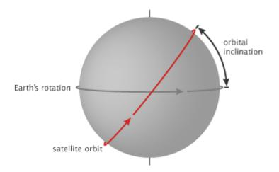
Orbital inclination is the angle between the plane of an orbit and the equator. An orbital inclination of  $0^{\circ}$  is directly above the equator,  $90^{\circ}$  crosses right above the pole, and  $180^{\circ}$  orbits above the equator in the opposite direction of Earth's spin. (NASA illustration by Robert Simmon.)
