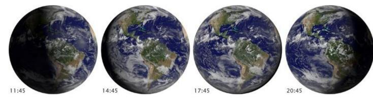
Satellites in geostationary orbit rotate with the Earth directly above the equator, continuously staying above the same spot. This position allows satellites to observe weather and other phenomena that vary on short timescales. (NASA images by Marit Jentoft-Nilsen and Robert Simmon.)
