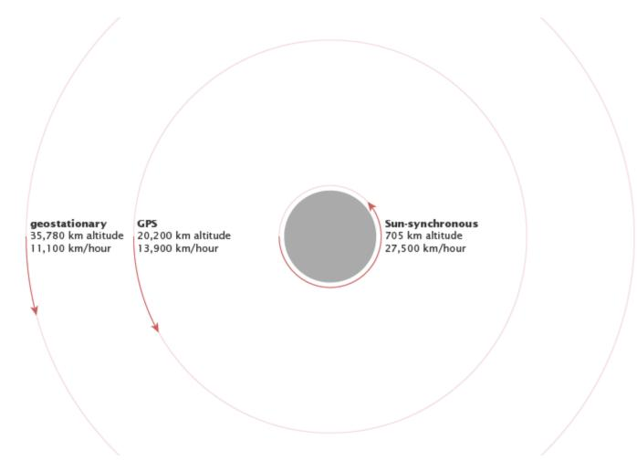
The higher a satellite's orbit, the slower it moves. Certain orbital altitudes have special properties, like a geosynchronous orbit, in which a satellite travels around the Earth exactly once each day. The length of each red arrow in this diagram represents the distance traveled by a satellite in an hour. <u>View animation</u>. (NASA illustration by Robert Simmon.)
