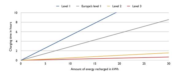
Figure 3:Time necessary for the charging process depending on the charging power and the amount of energy required.
