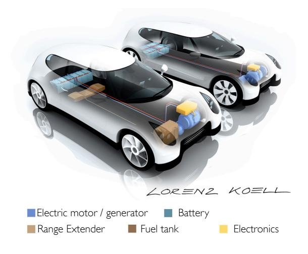
Figure 2: Hybrid car (left) and a pure electric car (right)
