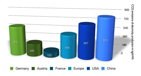
Figure 2: Specific emissions for electricity production in different countries<sup>2,3</sup>
