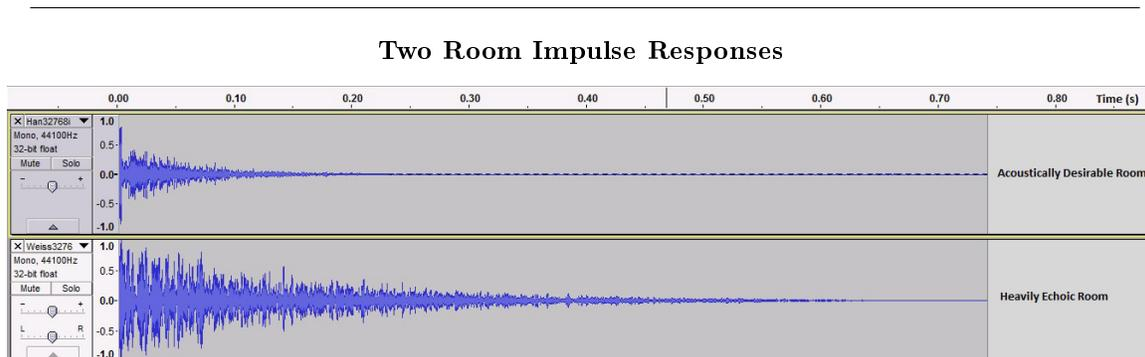
**Figure 2.1:** Echoes of the impulse can especially be seen in the echoic room, where the signal takes longer to decay.
