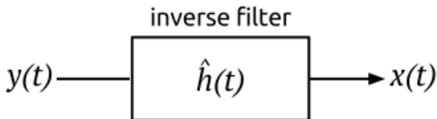
**Figure 3.2:** Inputting the echoed signal into the inverse filter yields the de-echoed signal.
