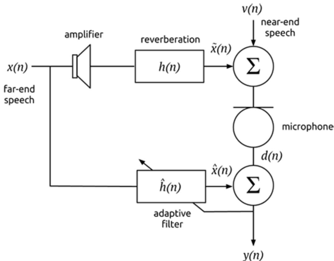
Figure 1.1: Block diagram example of typical acoustic echo cancellation.
