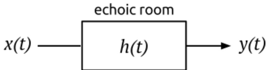
**Figure 3.1:** Block diagram of the echoic room as an LTI system with impulse response  $h(t)$  where  $y(t)$  is the echoed version of the input  $x(t)$ .
