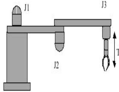
(b) Schematic of the SCARA RP41 mechanism
