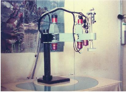
(a) The SCARA Robot RP41
