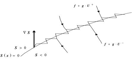
Figure 2. The geometric illustration of the sliding surface and switching of the vector fields on the hypersurface S(x) = 0
