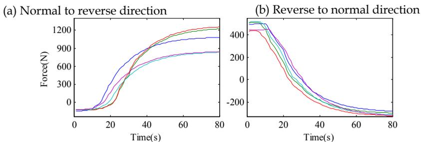
Fig. 2. Operating force curves for a point mechanism
