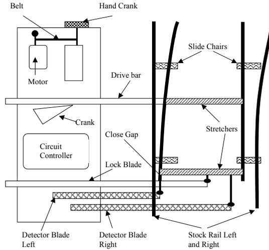
Fig. 1. Point Mechanism
