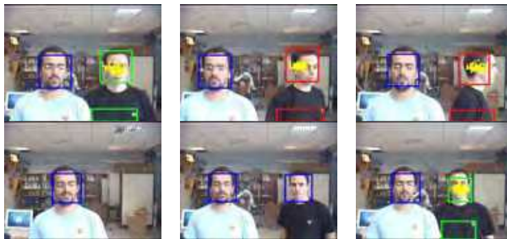
Figure 9. Tracking scenario including two persons with target out-of-sight. Target loss detection and automatic re-initialization
