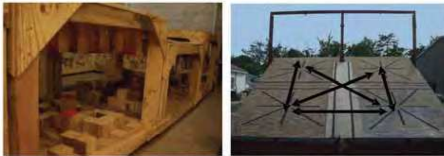
Fig. 3. Example Mobility Tests. Left: Confined Space Cubes; Right: Inclined Plane with waypoint pattern
