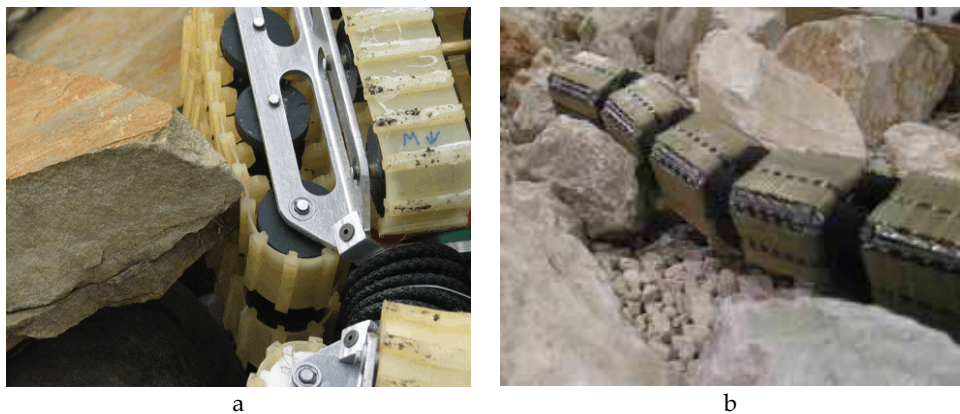
Fig. 5. Tracks all around: As the OmniTreads drive through rockbeds, it becomes apparent that side tracks help provide forward propulsion. a - OT-8; b - OT-4.
