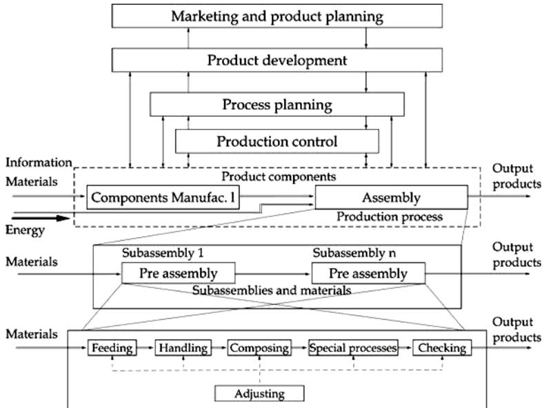
Fig. 3. Assembly as part of the production process (Rampersad, 1994)
