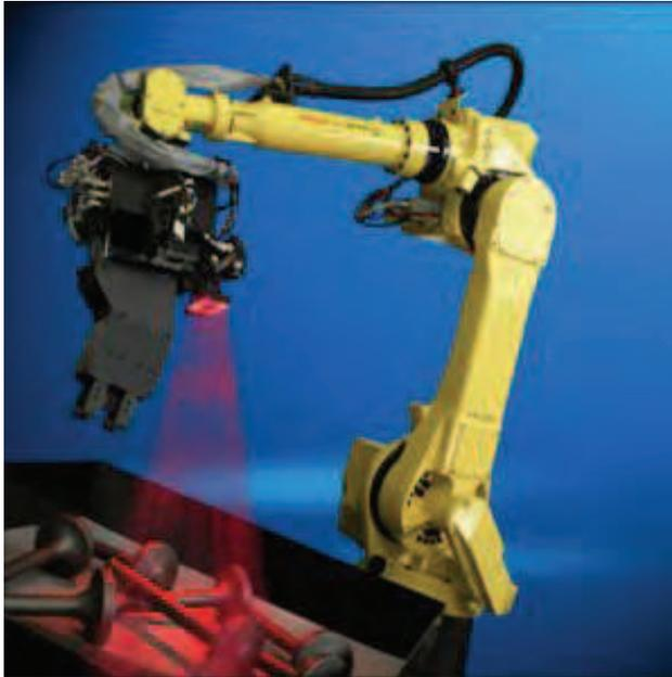
Fig. 2. Vision equipped robot in a bin picking application (Brumson, 2009)
