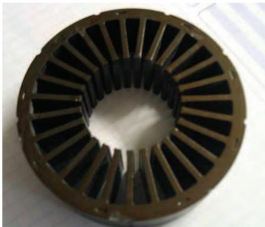
Fig. 8. EM stator assembled from thin metal plates
