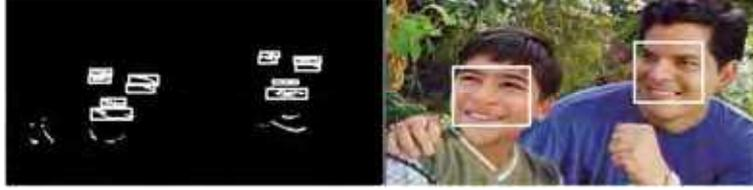
Figure 6. Results of Face Detection a) Facial Feature extraction b) Detected face in box
