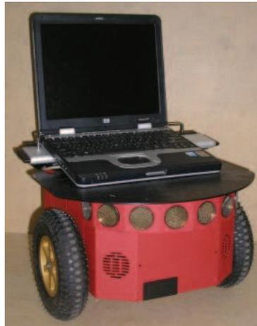
Figure 9. The Pioneer 3-DX robot with a laptop computer
