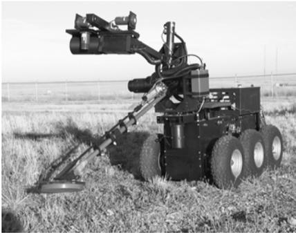
Fig. 5. Robotic Scanner mounted on teleoperated vehicle[5]
