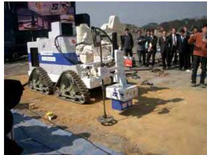
Fig. 8. Mine detection test of MHV
