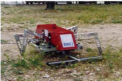
Fig. 3. Four legged mine detection robot
