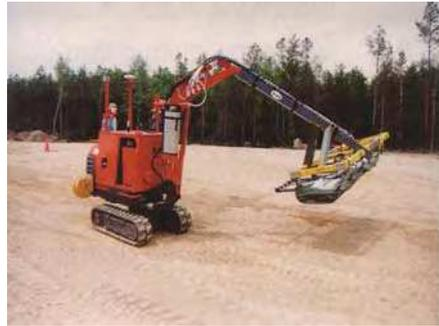
Fig. 6. Vehicle Mine Detector (VMMD)[6]
