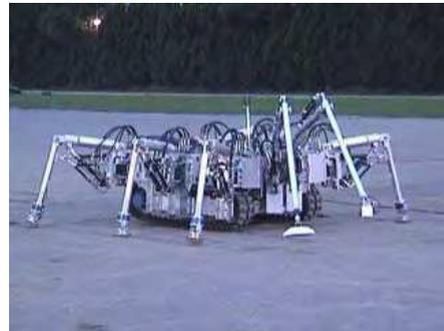
Fig. 4. Mine detection robot COMET-III
