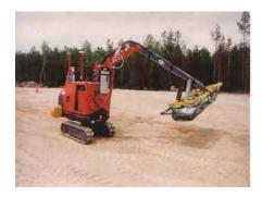
Fig. 5. Robotic Scanner mounted on teleoperated Fig. 6. Vehicle Mine Detector (VMMD)[6] vehicle[5]
