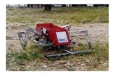
Fig. 3. Four legged mine detection robot
