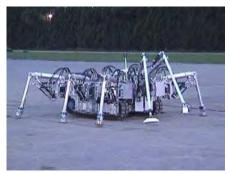
Fig. 4. Mine detection robot COMET-III
