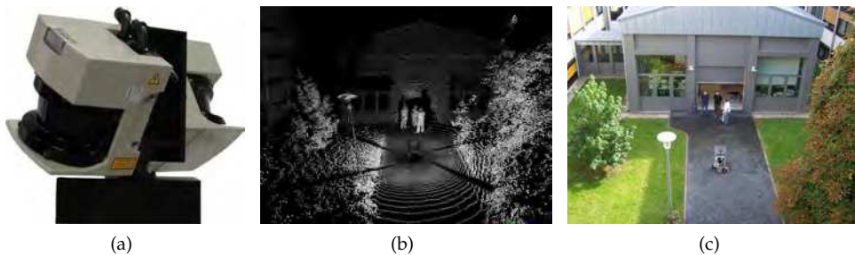
Fig. 3. Continuously rotating 3D laser scanner (a) and example data (b) taken in front of the Robotics Pavilion at Fraunhofer IAIS. A photo of the scene is shown in (c). The color of the 3D points in (b) corresponds to the received remission values.
