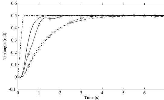
Fig. 9. Tip angle  $\theta_t$ : (—). Simulation with  $M_p = 0$ ; ( $\ominus$ ) Experiment with  $M_p = 0$ ; (---) Simulation with  $M_p = 0.3$ ; ( $\oplus$ ) Experiment with  $M_p = 0.3$ ; (---) the reference.
