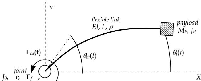
Fig. 1. Parametric representation of a single link flexible manipulator with a rotational joint.
