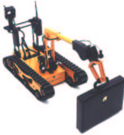
Figure 2.4: A vehicle with a high dimensional configuration space - a commercial bomb-disposal platform (picture courtesy of Roboprobe Ltd. The configuration space for a human is immensely high dimensional —around 230.
