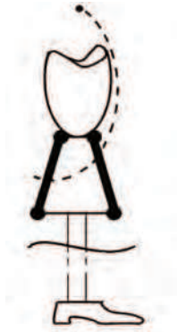
Fig. 5. Scheme of a four-axial mechanism for a prosthetic knee. The dotted line represents the path followed by the centre of rotation cr . The big dot represents the cr when the knee is extended. Placing this point more backward, results in a more stable stance phase
