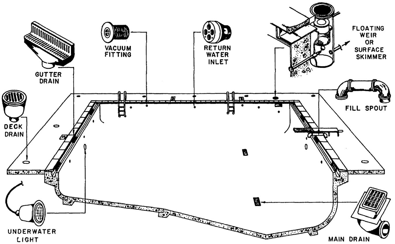
Figure 3-1. Longitudinal section through pool, showing fittings.
