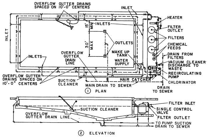
Figure 3-2. Typical recirculation pool and equipment. **3-3**
