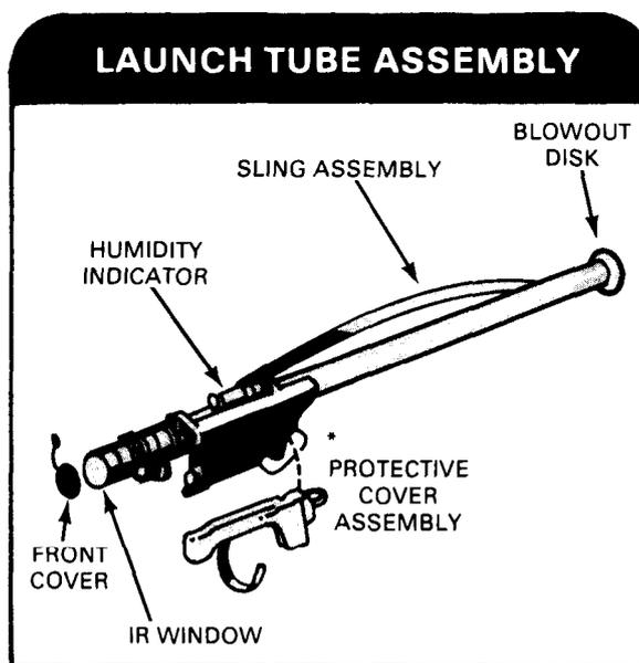
\*The protective cover assemblies should be retained for possible use in the event it becomes necessary to back pack weapons without the gripstock assemblies attached.
