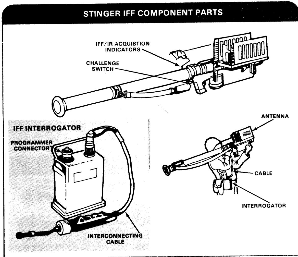
The gunner initiates the IFF sequence by pressing the IFF INTERROGATE switch on the gripstock assembly. Once the gunner issues a challenge, the rest of the sequence is automatic. The IFF interrogator, attached to the gunner's belt, sends a coded challenge (via an IFF antenna) to the aircraft. Aircraft
