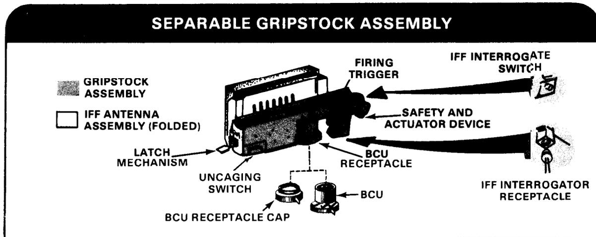
The antenna assembly folds into a holder on the right side of the gripstock assembly when not in use. When it is deployed and the interrogator is connected to the gripstock, it is capable of interrogating aircraft and
