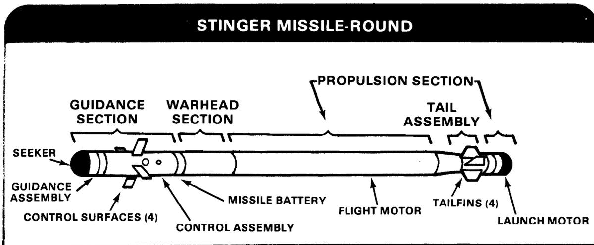
The guidance section of the missile consists of a guidance assembly, a control assembly, a missile battery, and four control
