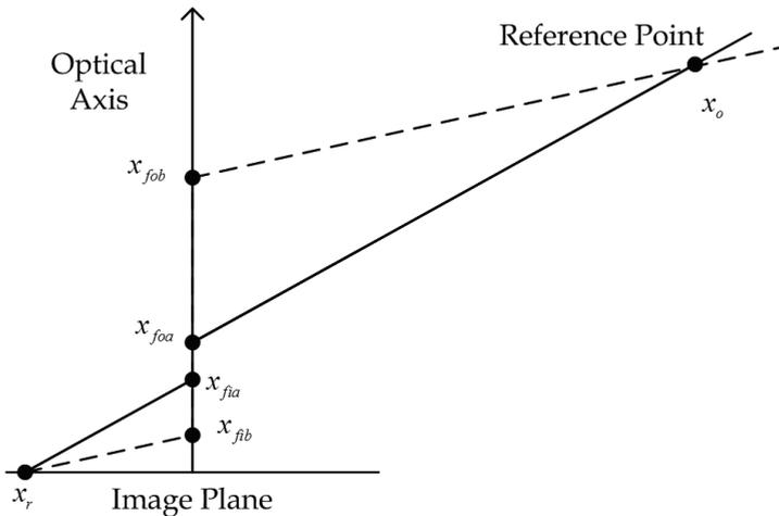
Fig. 7. If the distance to the reference does not vary two different sets of camera parameters  $a$  and  $b$  can both give a small error norm in both image and object space. The calibration can not determine if situation  $a$  or the dotted  $b$  in the figure is the right one.
