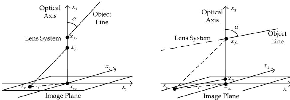
Fig. 3. Geometrical construction of the GCM, with different inclination angles. The points  $x_{fo}$  and  $x_{fi}$  can slide along the optical axis depending on  $r$ , the distance to the centre principal point. For large angles,  $\alpha$ , the undistorted image point of the CCM would be far away from the centre of the image, causing problems for the CCM. The GCM solves that by having  $x_{fi}$  close to the detector (or even below it).
