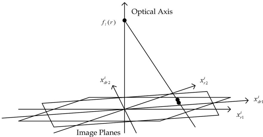
Fig. 4. The leaning image compensation converts between leaning and non-leaning detectors so that a line between the points on the two planes hits the optical axis at a point  $f_i(r)$  units from the principal point.
