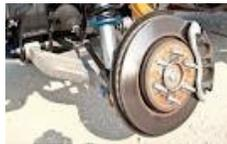
I cleaned the whole caliper and slide mechanism to ensure it would operate correctly. I replaced the cracked disc with a genuine Ford disc. After re-assembling the brakes, I pumped the brake pedal until it was hard. The hub was now free to spin by hand.
