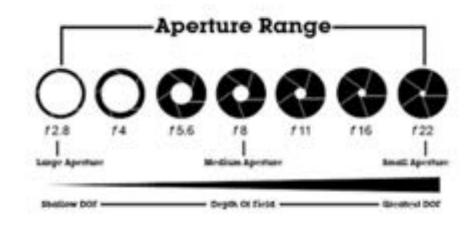
DEPTH OF FIELD IS EFFECTED BY THE APERTURE. THE BIGGER THE HOLE (SMALLER THE NUMBER) A SMALLER AMOUNT WILL ABLE TO BE IN FOCUS. AND VICE VERSA, THE SMALLER THE HOLE (BIGGER NUMBER) THE MORE OF YOUR IMAGE WILL BE IN FOCUS.
