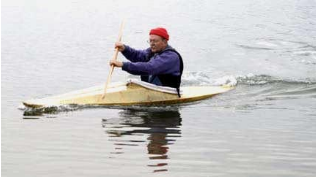
Note how both the bow and the stern create waves as this displacement hull moves through the water.
