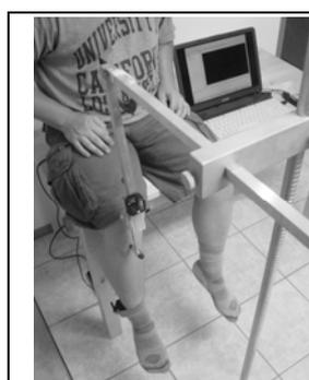
Fig. 2. Third generation wireless accelerometer reflex quantification device
