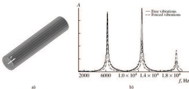
Fig. 8. (a) Model of a thin rod and (b) calculated spectra of free and forced vibrations in the rod.
