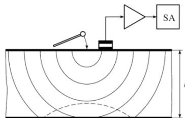
Fig. 1. Schematic diagram of testing of a flaw-free concrete article ( $h = 0.5$  m) by the acoustic IE method.
