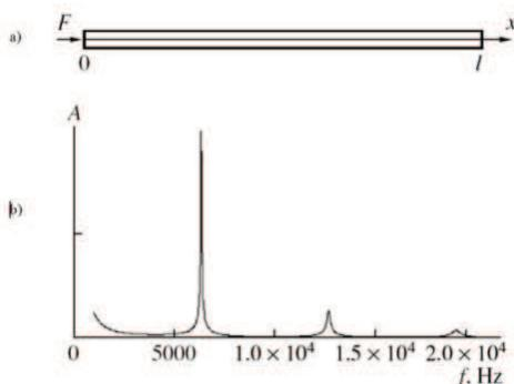
Fig. 7. (a) Thin concrete rod and (b) spectrum of forced vibrations in the rod.
