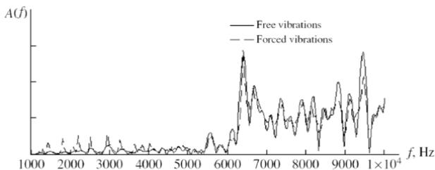
Fig. 10. Spectra of free and forced vibrations for a slab with dimensions of 300×300×30 cm.
