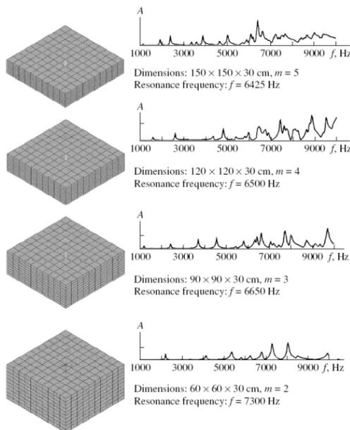
Fig. 12. Spectral characteristics of a compact slab with a thickness of 30 cm at different values of the compactness  $m$ .
