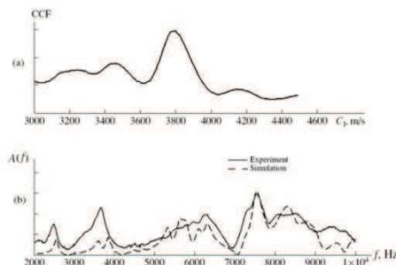
Fig. 14. (a) Dependence of the CCF on the velocity and (b) coincidence of the experimental and calculated spectral characteristics.
