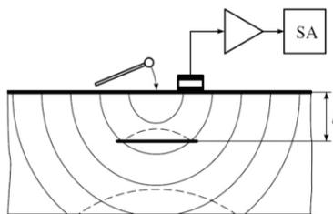
Fig. 3. Schematic diagram of testing of an extended concrete article ( $h = 0.5$  m) with a flaw ( $l = 0.25$  m) by the acoustic IE method.
