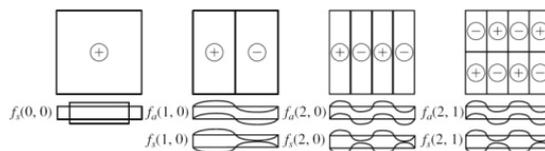
Fig. 11. Some forms of flexural and planar vibrations in a plate.
