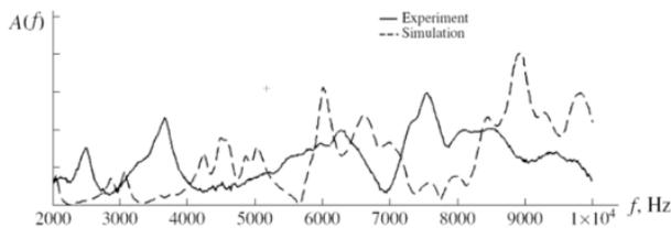
Fig. 13. Experimental and calculated spectral characteristics for a block with dimensions of  $80 \times 50 \times 30$  cm (simulation at  $C_1 = 3000$  m/s).
