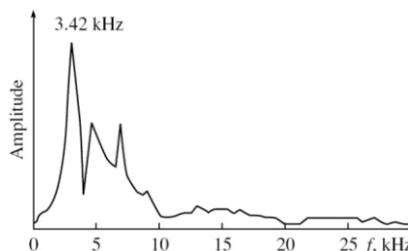
Fig. 2. AFC of an extended flaw-free concrete article:  $f = 3.42$  kHz and  $h = C / 2f = C\lambda / 2$ .
