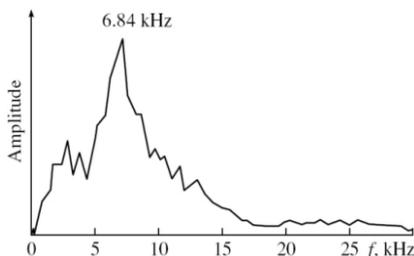
Fig. 4. AFC of an extended concrete article with a flaw:  $f = 6.84$  kHz and  $l = 0.25$  m.
