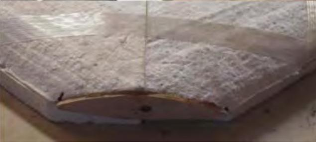
Front of wing is then cut off (no incidence up or down, thrust right or left). Plywood motor mount/firewall with 3" dowel is epoxied on (with 30minute Mercury Adhesive).
