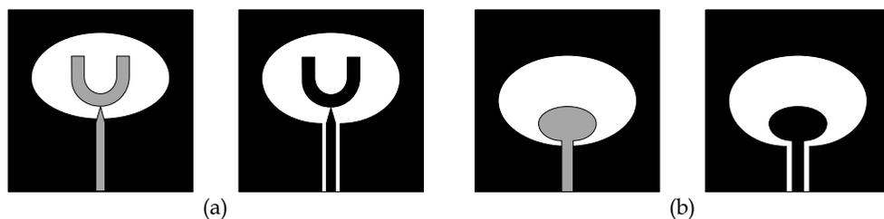
Fig. 17. The Microstrip-fed / CPW-fed UWB slot antennas
