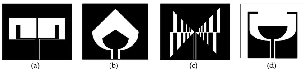
Fig. 16. The UWB slot antennas using CPW feeding line
