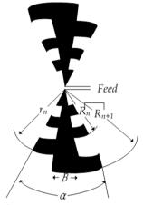
Fig. 5. The logarithmically periodic antenna structure
