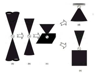
Fig. 7. Evoluation processes from the conical antenna to disc cone antenna and planar monopole antenna
