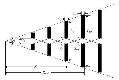
Fig. 6. The log-periodic dipole antenna geometry
