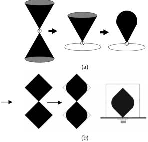
Fig. 8. The modified bowtie antenna structures
