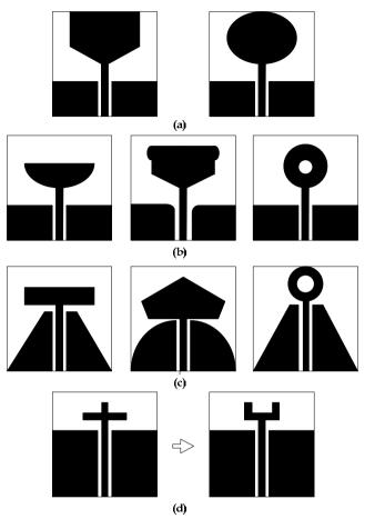
Fig. 14. The CPW-fed monopole UWB antennas
