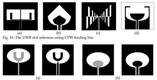
Fig. 17. The Microstrip-fed /CPW-fed UWB slot antennas
