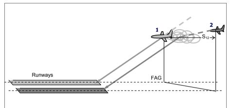
horizontal and vertical separation rules simultaneously. Figure 4 (a, b) shows the principal difference between CNAP and SEAP performed under IMC (Janic, 2008a).
