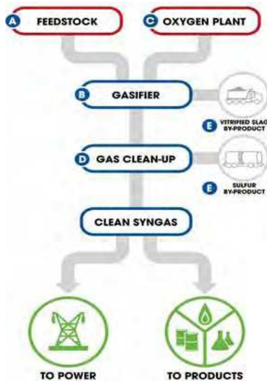
Fig. 7. A schematic diagram of gasification process
