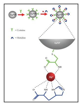
Fig. 2. Schematic representation of colorimetric sensor for histidine determination.
