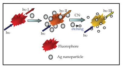
Fig. 3. Schematic representation of AgNPs-cyanide determination by IFE.
