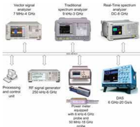
Fig. 3. Measurement station for performance assessment.
