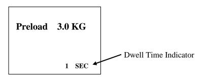
4. After the dwell time elapses, the indenter automatically resumes moving and applies more force until the force reaches the load force. Then, the indenter stops
