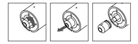
Then pull out the sleeve and replace the indenter with the correct one:
