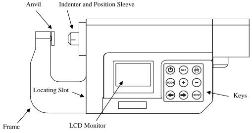
Fig. 1: Tester Front View
