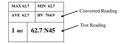
Finally, the LCD monitor will display the test reading:
