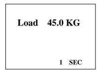
5. After the pause, the indenter automatically moves backwards and decreases the force it applies on the test specimen until the force decreases back to the preliminary test force. Then the indenter stops moving and pauses for a specified dwell time. The LCD monitor displays this screen:
