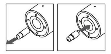
Reinsert the sleeve and twist to lock the sleeve:
