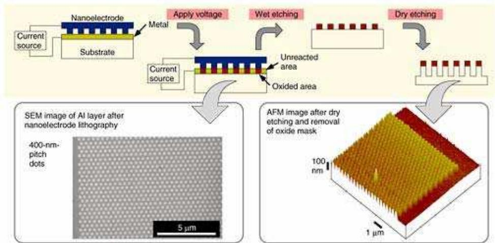
Fig. 8. Chemical nanoimprint (nanoelectrode lithography) (Yokoo & Namatsu, 2009)
