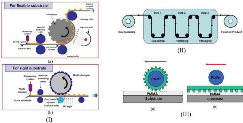
Fig. 7. Roller-type Nanoimprint Lithography (Lan et al., 2008)
