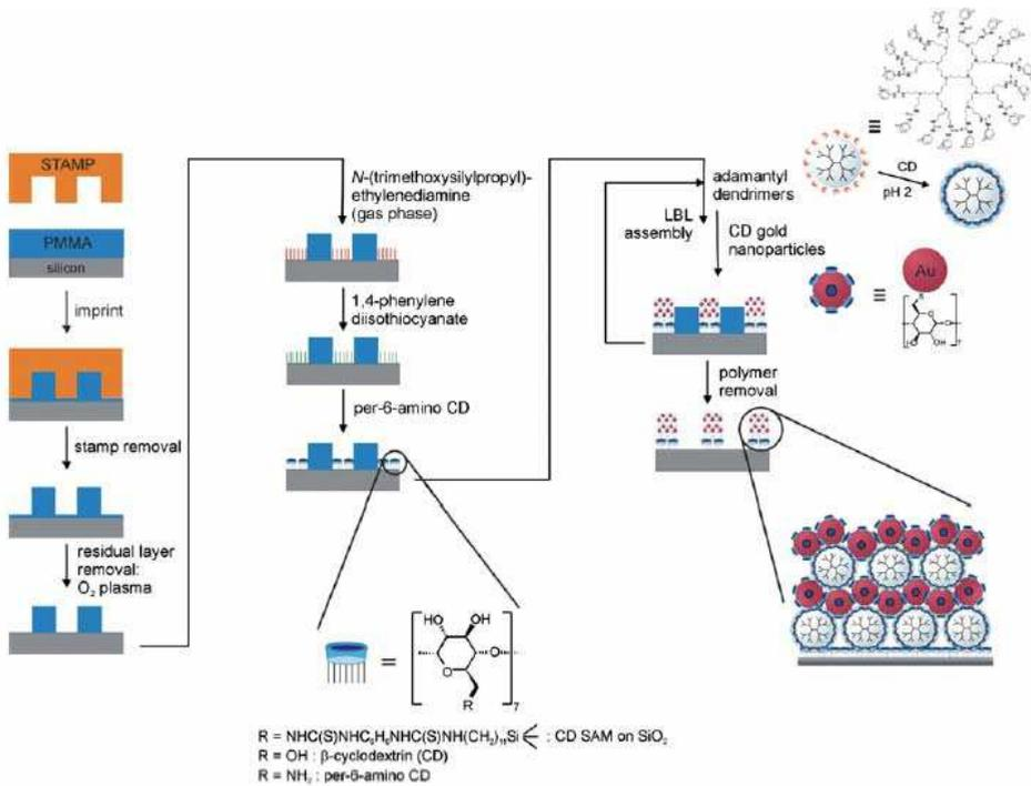
Fig. 9. Integrated nanofabrication scheme on nanoimprinted pattern (Plachetka et al., 2008)
