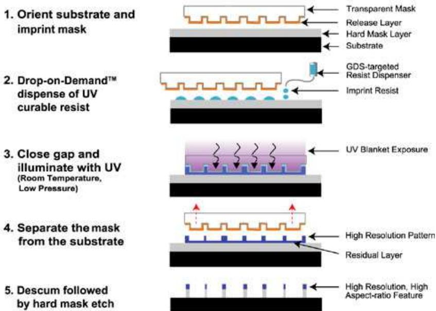
Fig. 3. Jet and Flash™ imprint lithography process (J-FIL, 2009)
