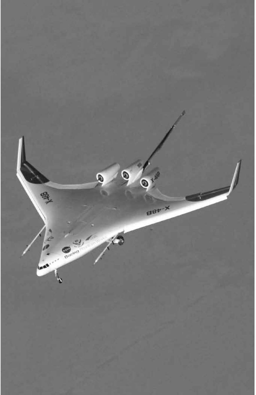
The X-48B subscale demonstrator for the Blended Wing-Body (BWB). The BWB may represent the next extension of the swept and delta wing, to transform flight away from the rule of the "tube and wing" jetliner. NASA.
