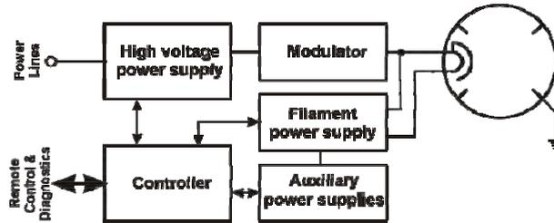
Fig. 6. Block-diagram of magnetron transmitter.
