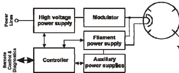
Fig. 6. Block-diagram of magnetron transmitter.
