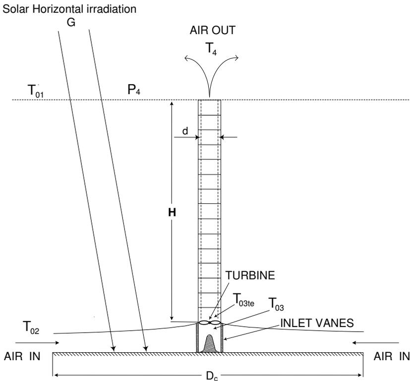
Fig. 4. Schematic diagram of the SAEP in operation
