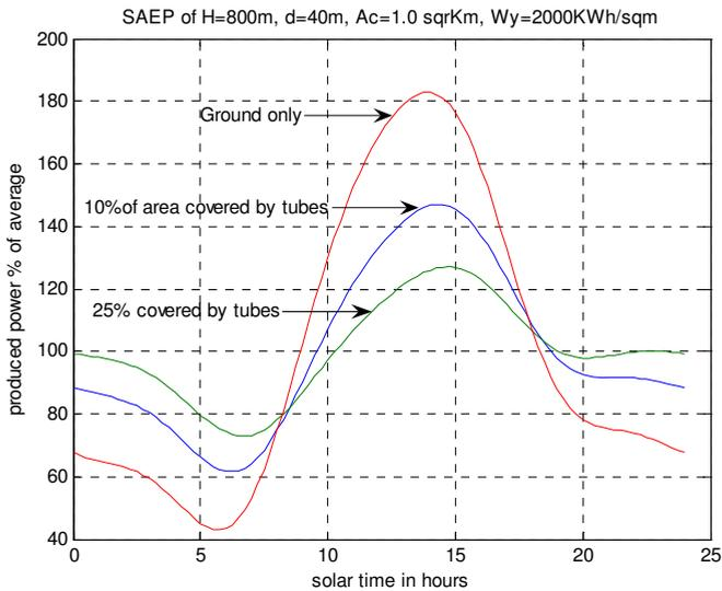
Fig. 13. The average daily SAEP’s electricity generating profiles
