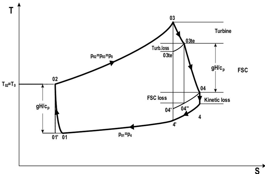
Fig. 7. The thermodynamic diagram of the SAEP
