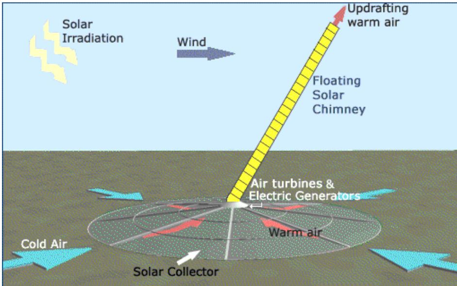
Fig. 1. Floating Solar Chimney Power Plant in operation
