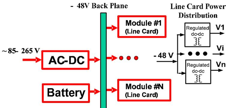
Fig. 4. Example of distributed power architecture
