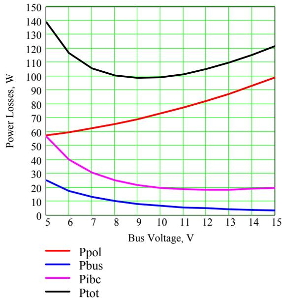
Fig. 7. Power losses over bus voltage
