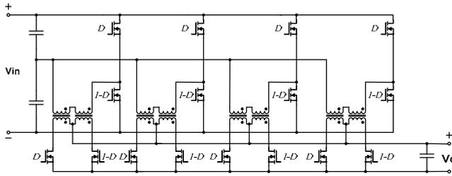
Fig. 10. Four phases interleaved asymmetrical half-bridge.
