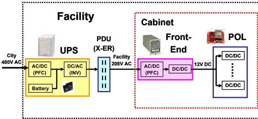
Fig. 1. Typical power system of data center
