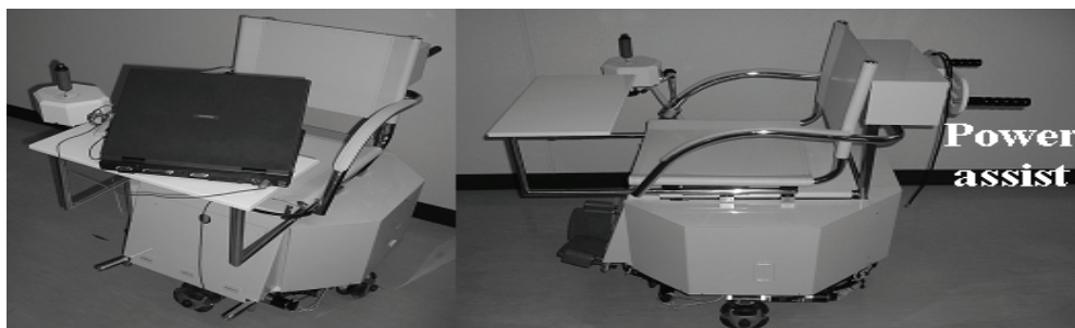
Fig. 1. Omni-directional wheelchair (OMW)
