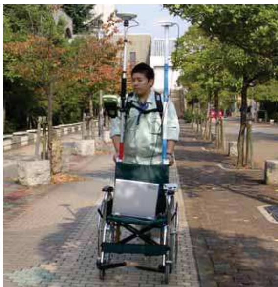
Fig. 4. Positioning of D-GPS and VRS-GPS
