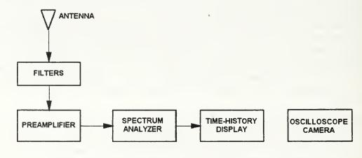
Figure 1 Block Diagram of the Instrumentation
