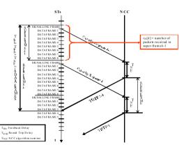
Fig. 2. DAMA algorithm: TBTP computed from RCST requests
