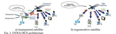
Satellite Terminals (RCST) provide single PC or LANs with the access to the network, while Gateways (GWs) allow the connection with Internet core networks. The uplink access from each RCST is managed through DVB-RCS interfaces.
