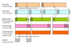
Fig. 3. GSE encapsulation in DVB-S2
